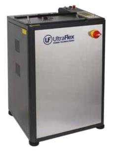
SuperCast J is the most advanced universal casting machine on the market which utilizes the patented Rotating Coil System (RCS). The RCS continues to melt the metal while spinning and injecting. This way the system maintains the molten metal's viscosity during casting and prevents premature solidification due to coil lifting and injection delays. This unique feature guarantees perfect casting results with high-temperature, fast solidifying metals such as Platinum, Palladium and Titanium.
